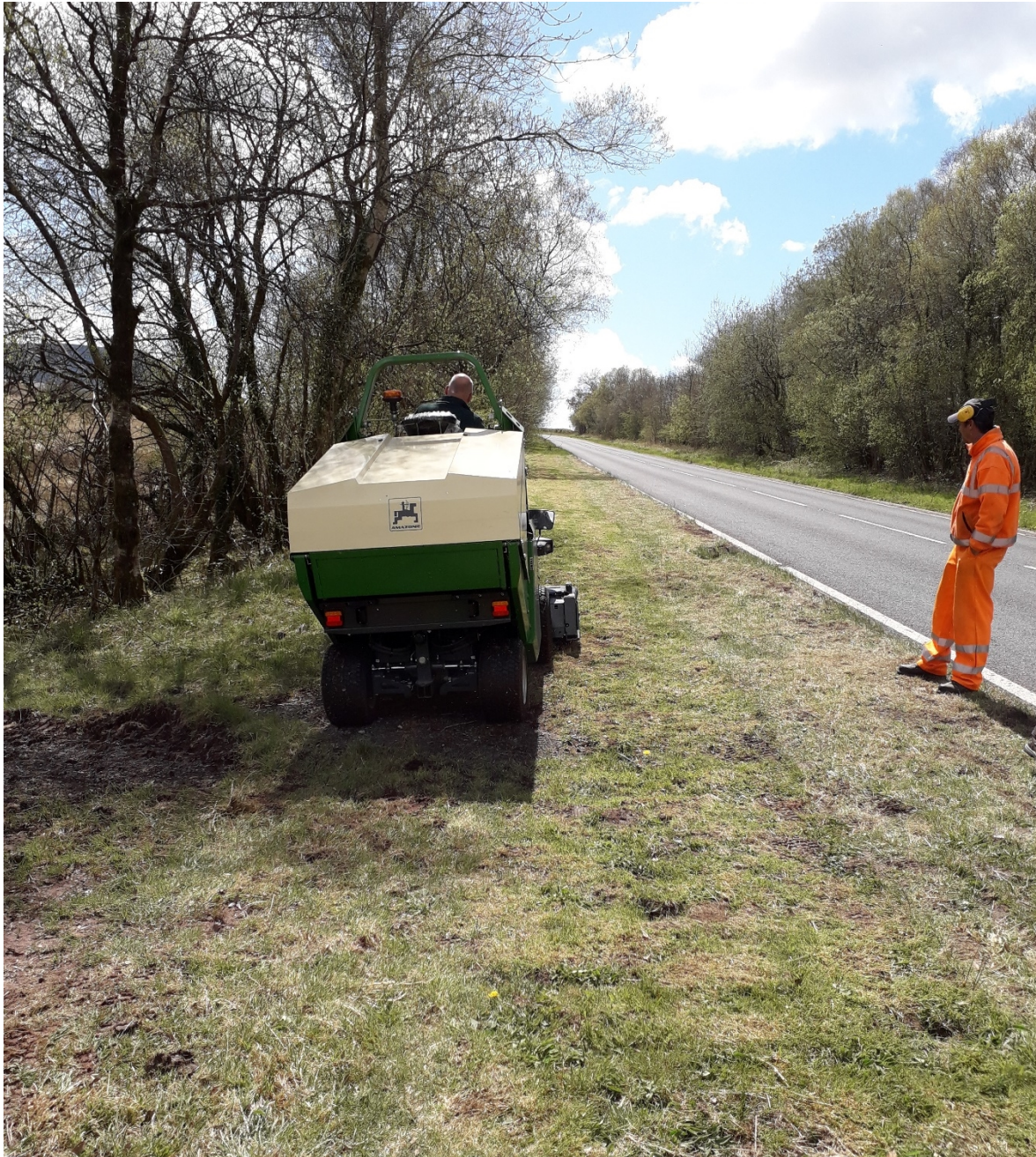
FIGURE 2.1: CUT & COLLECT MACHINE USED BY HIGHWAYS TO MANAGE ROADSIDE VERGE NATURE RESERVES (RVNRs).
